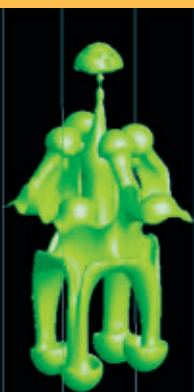
>>> A heavy fluid is superimposed on a lighter one in a vertical square duct. Under the effect of gravity both fluids mix together: the heavy fluid flows down (preferentially near the corners), while the lighter one flows up (preferentially in the core of the duct). The image shows the boundary of the mixed zone at a given instant, represented by the surface on which both fluid phases are present in the same concentration.
