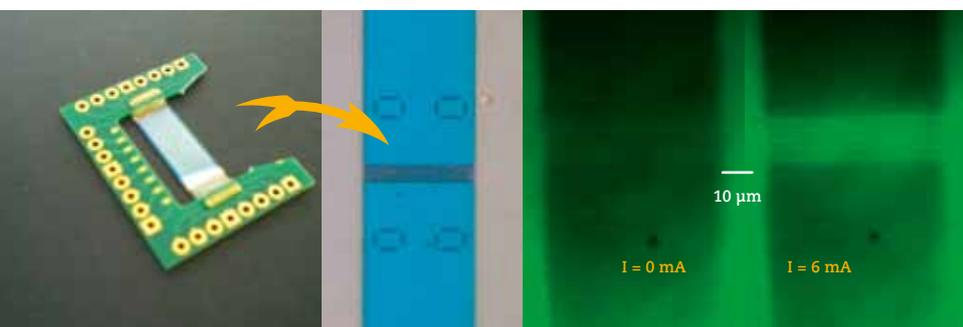
>>> Electronic device including nickel microwires covered by fluorescent doped spin crossover Nps before (low spin state) and after (high spin state) the application of a bias of 6mA. Clearly, the fluorescence intensity of the fluorophore is modulated by the spin state of the material.
