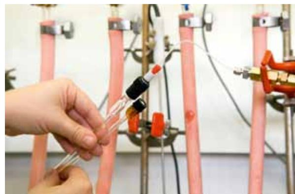
>>> Pressure NMR tube (NMR = Nuclear Magnetic Resonance) for in situ monitoring of the catalyzed hydrogenation of benzonitrile.
