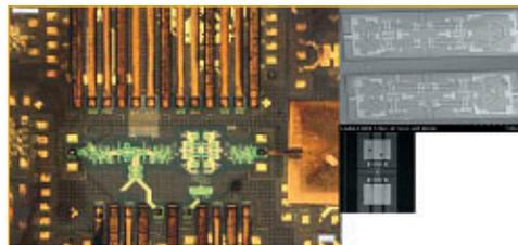
>>> 3D architecture of reconfigurable millimetre-sized communication system composed of a silicon integrated circuit (developed by the University of Toronto and made by ST Microelectronics), an electromagnetic transducer and a miniaturized antenna.
