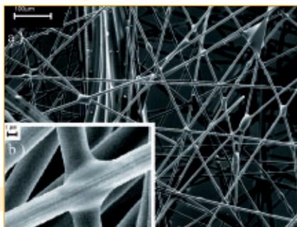
>>> a) Tangled, reticulated material for sandwich structure core made with carbon fibres, volumic mass 180kg/m<sup>3</sup>, b) zoom on an epoxy graft
