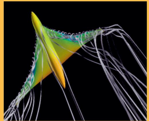
>>> Direct numerical simulation of the flow around the epistle at high angle of attack ©Onera
