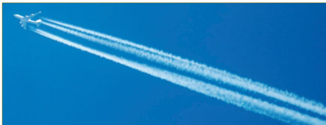
>>> Aeroplane trail with ice particles transported in the vortices created around the wing
