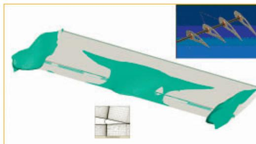
>>> Negative take off speeds behind a wing with aileron, and morphing schematic.
