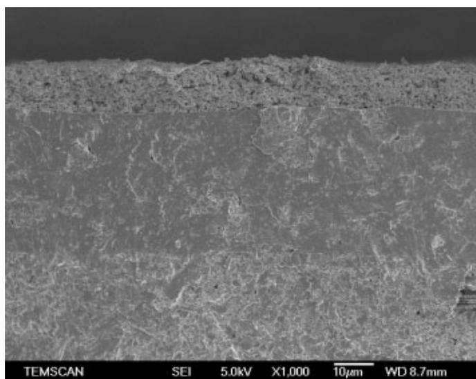
>>> Micrograph of an anode-supported SOFC mono-cell
