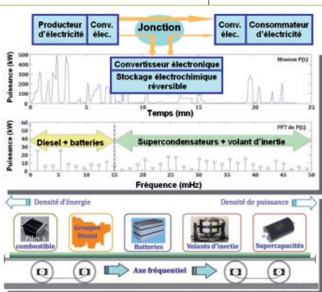
>>> Illustration of frequency sharing of powers provided by different sources in the hybrid locomotive LHYDIE and of the power flows in a generic hybrid junction (from R. Akli, X. ROBOAM, B. Sareni).
