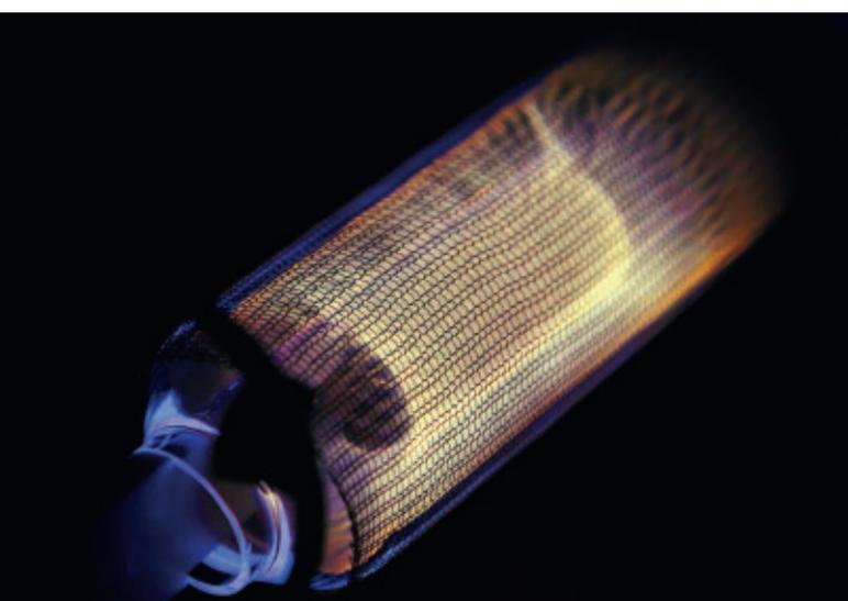
>>> Dielectric Barrier Discharge lamp produced at LAPLACE. This lamp uses a novel concept for light generation: molecular radiators, which might even be the next generation of light sources.
