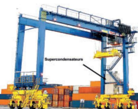
>>> A supercapacitor integrated into a crane.
