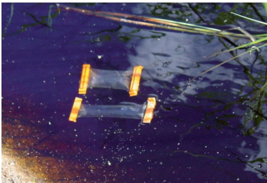
>>> Dialysis experiment to recover the colloidal fraction of marshy water particularly rich in organic matter and iron oxides (from Karelia region, Russia)
