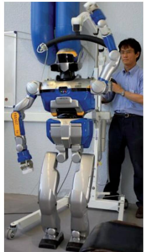
>>> HRP-2: 1,54m, 58kg, 30 degrees of freedom, 4 cameras, 4 force sensors, 1 gyroscope, 1 accelerometer
