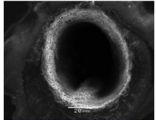
>>> Laser ablation in a sample of Monazite (Brazil). Energy: 100 microjoules/pulse, pulse width: 100fs, rate: 5Hz, duration: 120s. Note the sharp edges and walls of the crater, and the absence of melt.
