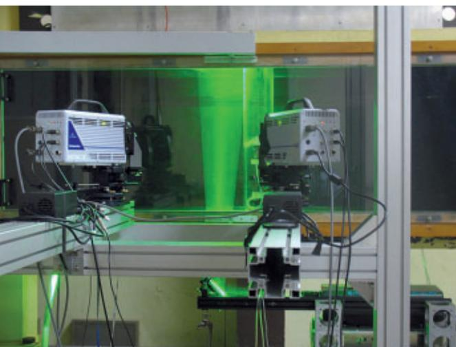
>>> Time Resolved Stereoscopic PIV measurements in the near wake of a circular cylinder in IMFT's wind tunnel.
