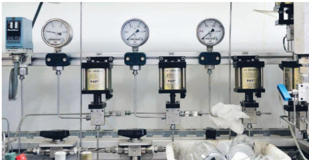
>>> Pilot micro-unit of methanol carbonylation to acetic acid.
