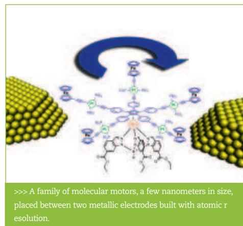
>>> A family of molecular motors, a few nanometers in size, placed between two metallic electrodes built with atomic resolution.
