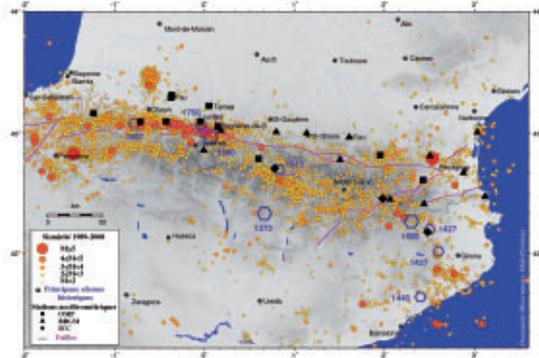
>>> Accelerometric network of the Pyrenees, superimposed on the instrumental seismicity since 1989, and to main historical events.
