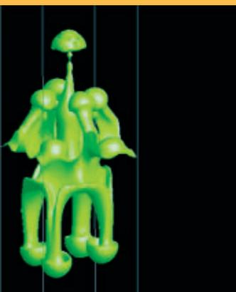
>>> A heavy fluid is superimposed on a lighter one in a vertical square duct. Under the effect of gravity both fluids mix together: the heavy fluid flows down (preferentially near the corners), while the lighter one flows up (preferentially in the core of the duct). The image shows the boundary of the mixed zone at a given instant, represented by the surface on which both fluid phases are present in the same concentration.
