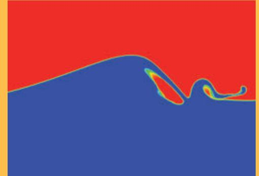
>>> Simulation of a Stokes wave plunging in deep water performed with JADIM (in-house code)
