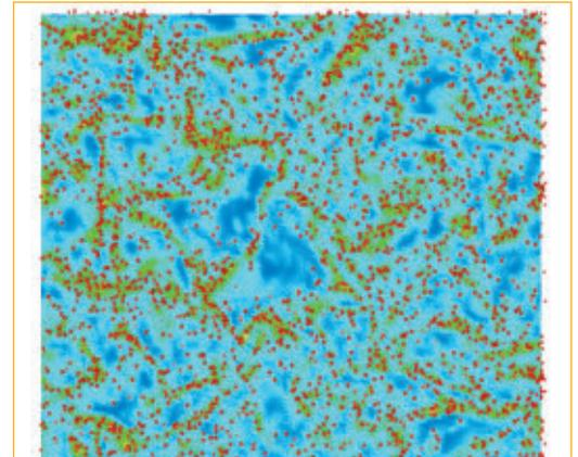
>>> Snapshot extracted from a 3D simulation of a droplet cloud evaporating in hot turbulent air. (The coloured portion corresponds to the fuel vapour field).
