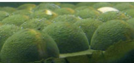
>>> artificial substrates in a hydraulic channel turbulent flow at the IMFT, covered by a growing river biofilm.
